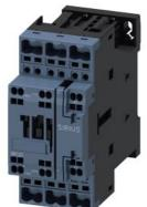
power contactor, AC-3e/AC-3, 12 A, 5.5 kW / 400 V, 3-pole, 24 V AC, 50/60 Hz, auxiliary contacts: 1 NO + 1 NC, spring-loaded terminal
