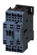
power contactor, AC-3e/AC-3, 12 A, 5.5 kW / 400 V, 3-pole, 24 V AC, 50/60 Hz, auxiliary contacts: 1 NO + 1 NC, spring-loaded terminal, upright mounting position
