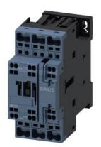
power contactor, AC-3e/AC-3, 12 A, 5.5 kW / 400 V, 3-pole, 110 V AC, 50 Hz, auxiliary contacts: 1 NO + 1 NC, spring-loaded terminal
