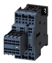
power contactor, AC-3e/AC-3, 12 A, 5.5 kW / 400 V, 3-pole, 110 V AC, 50 Hz, auxiliary contacts: 2 NO + 2 NC, spring-loaded terminal, removable auxiliary switch
