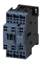
power contactor, AC-3e/AC-3, 12 A, 5.5 kW / 400 V, 3-pole, 220 V AC, 50/60 Hz, auxiliary contacts: 1 NO + 1 NC, spring-loaded terminal
