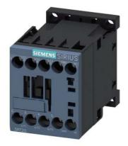
power contactor, AC-3e/AC-3, 9 A, 4 kW / 400 V, 3-pole, 400 V AC, 50/60 Hz, auxiliary contacts: 1 NO, screw terminal
