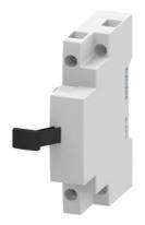
Undervoltage release 415 V AC/50 Hz, 480 V AC/60 Hz with leading auxiliary switch 2NO, for circuit breaker 3RV1011
