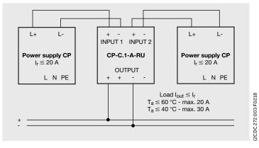
True redundancy using a CP-C.1-A-RU redundancy unit
