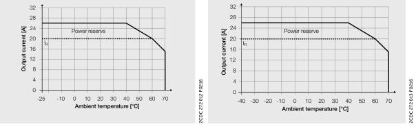
Characteristic curves of temperature at  $U_{\rm out}$  = 24 V, mounting position 1
