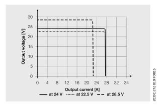
Characteristic curve of output at Ta = 25  $^{\circ}\mathrm{C}$
