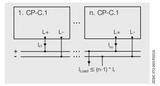
Simple redundancy or n+1 setup
