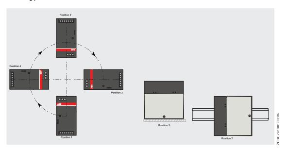
In order to ensure a sufficient convection in mounting position 1 and 7, the minimum distance to other modules must not be less than 25 mm in vertical direction and 25 mm in horizontal direction. For the derating of the output current, see the characteristic curve of temperature. Details for other mounting positions on request.
