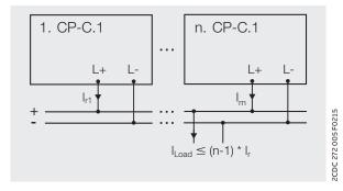
Simple redundancy or n+1 setup
