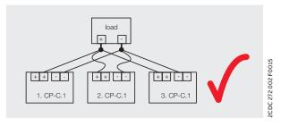
Correct wiring for increased power
