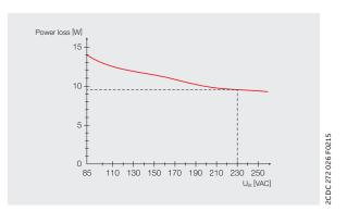
Typical efficiency over AC input voltage
