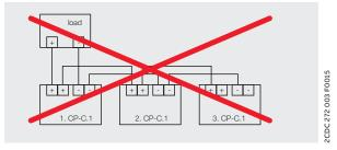
Incorrect wiring for increased power
