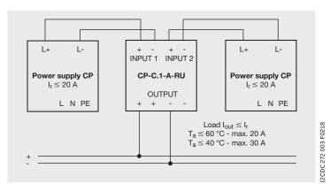
True redundancy using a CP-C.1-A-RU redundancy unit
