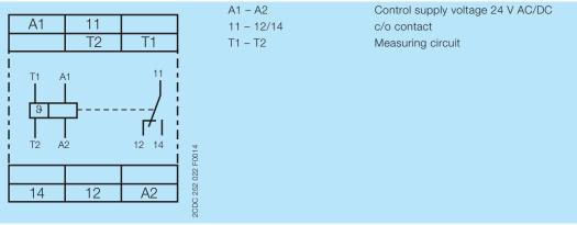
Connection diagram CM-MSS.12
