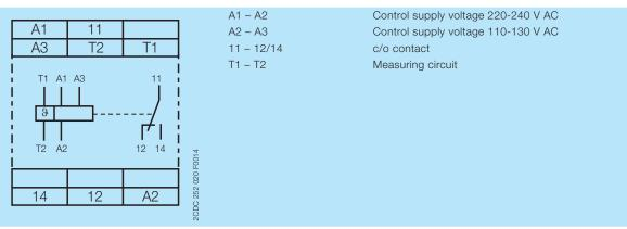
Connection diagram CM-MSS.13
