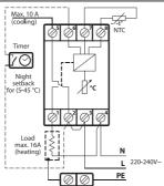
The screen of the heating cable must be connected to the earth conductor of the power supply cable by using a separate connector.
