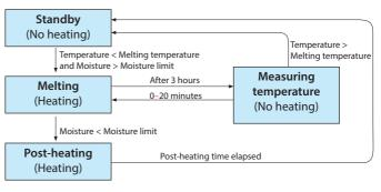
manual). By combining measurements of both moisture and temperature a reliable detection of the situation is achieved. Hence it is known whether heating of the roof area is needed in order to avoid that the roof is covered by ice and snow.
