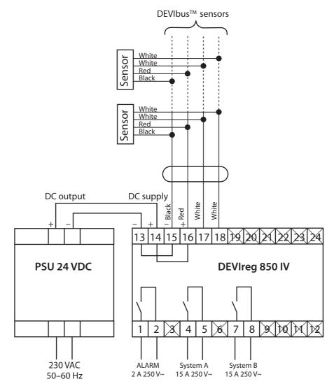
The DEVIreg<sup>™</sup> 850 has an integral alarm function that monitors the attached sensors and the in-built microprocessor.
