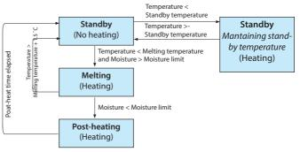
bining measurements of both moisture and temperature a reliable detection of the situation is achieved.
