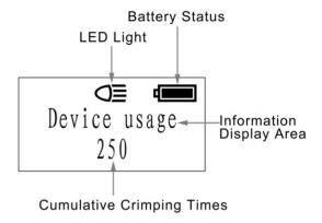
Tool LED illuminator: After clicking the start button, the LED illuminator lights on, After the tool is released, the button will automatically turn off after a delay of 20 seconds. Press the start button before installing the battery. When the battery is installed, release the start button and the LED light is off. If the light is on, the battery must be reinstalled once. As shown in the figure.
