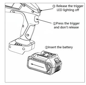
installed, release the start button and the LED light is off. If the light is on, the battery must be reinstalled once. As shown in the figure.
