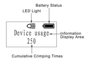
Tool LED illuminator: After clicking the start the LED button, illuminator lights on, After the tool is released, the light will automatically turn off after a delay of 20 seconds. Press the start button before installing the battery. When the battery is
