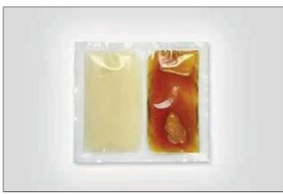
Two-component polyurethane cast resin PUR 112 FR.
