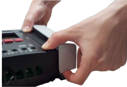
Fig. 3: Release the cover from the end position (here the right cover)
