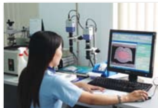
Crimp cross sectioning analysis equipment
