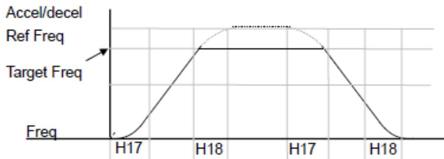
**Note:** If Target Frequency is below Max Frequency, the waveform will be shown with the top portion cut out.
