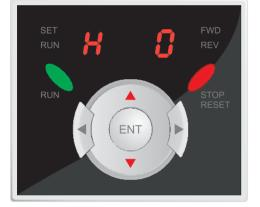
7.2 Use the up and down arrows on the navigation pad to move between parameters within the selected parameter group.
