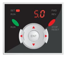
7.4 Use the left and right arrows on the navigation pad to move between digits. Use the up and down arrows to increase or decrease the digit value.
