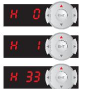
In this example, we will set Parameter H33 (Function Group 2 "H", Parameter number 33) which is motor rated current.
