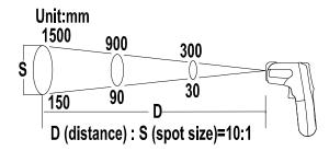
Make sure that the target is larger than the meter's visual spot size. The smaller the target, the closer you should be to it. The relationship between distance and spot size is 10:1
