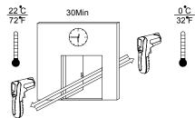
**Note2** When ambient temperature changes quickly, must wait 30 minutes to balance the temperature of the instrument before use.
