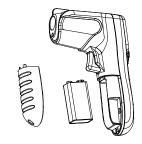
**Note3** When the battery voltage is lower, the battery symbol appears, it indicates that we must change the battery
