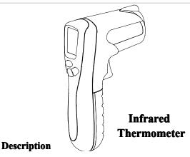
Noncontact Themometer detects the infrared ray that an object emits, The instrument foculizes infrared energy of the object onto a sensor through a lens, changes the surface temperature into electric signal, calculates microcomputer and displays the measurement temperature on the LCD.
