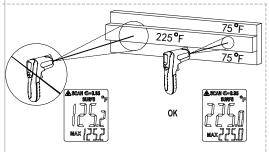
**Note1** Make sure that the target is larger than the meter's visual spot size
