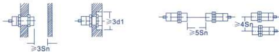
S_n is the detection distance, d_1 is the diameter of sensing surface.
