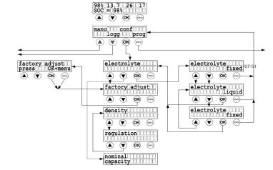
enter the electrolyte setting window and you may toggle between the settings "fixed" and "liquid" by pressing the arrow keys ▲ ▼. After having selected the desired configuration, press **OK** to confirm the configuration. Now you are free to either enter further windows by pressing the arrow keys ▲ ▼ or to get back to the main menu by pressing the menu key. 5.8.3 Reset to Factory Pre-Set Configuration
