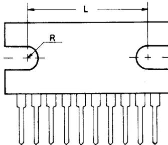
3. The screw to be used must have a head equivalent to the truss machine screw or binder machine screw defined by JIS. Washers must be also used to protect the IC case.
