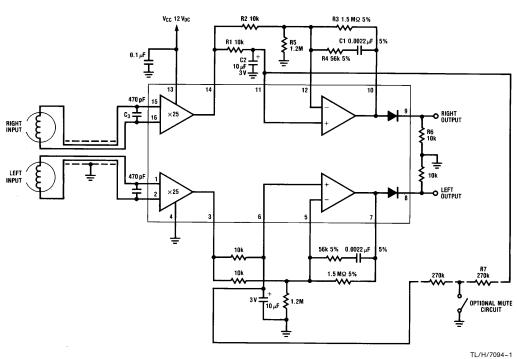
FIGURE 1. Typical Tape Playback Preamplifier Application
