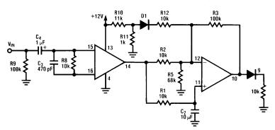
FIGURE 9. Microphone Preamplifier with Capacitor Coupled Input
