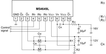
CM : Capacitor for noise absorption when the motor rotates. Use the IC with CM set to  $0.1\mu F$  or less.
