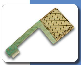
TwinSenZ sensors are a combination of IEE's capacitive and FSR technologies.
